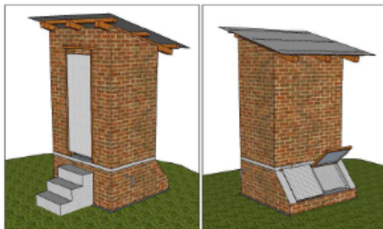
3D image of an ECOSAN latrine (PAD)
